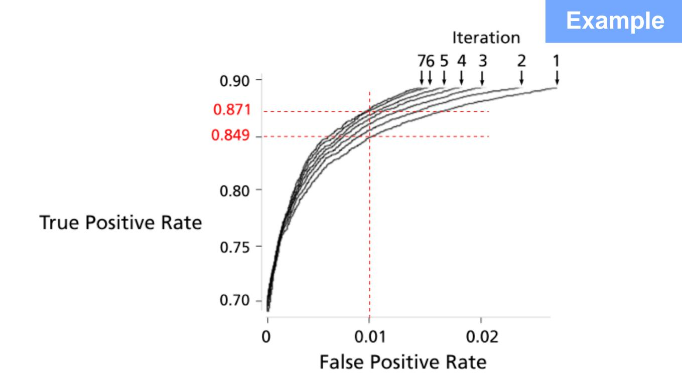
Figure 8: ROC curves of 7 iterations; true positive rate incrementally improves.
