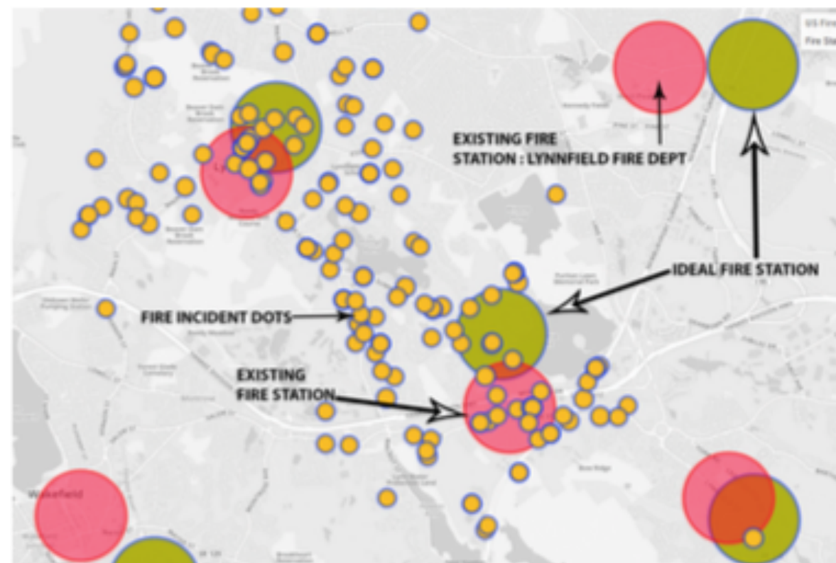
Figure 1: Screenshot of ISPARK showing actual (pink) and predicted (green) fire station locations in Maine determined by our approach, using coordinates with actual driving distances from fire stations to actual fire incidents. Fire incidents are shown as small yellow dots. ISPARK reduces the average
